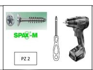
IMPORTANT NOTE: PLEASE HALF TIGHT THE SCREWS DURING THE ASSEMBLY. AFTER FINISHING THE ASSEMBLY FULLY TIGHT THE SCREWS
