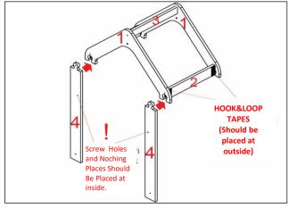
PLEASE PASS ON THE OTHER SIDE, PLACE THE SHELVES(CODE:5) AND BOTTOM RAILS(CODE:3 WITHOUT HOOK &LOOP TAPES) INTO THE SIDE STRUTS' NOTCHES(CODE4:) AND THEN TIGHTEN THE SCREWS.
