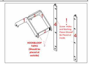
PLEASE PASS ON THE OTHER SIDE, PLACE THE SHELVES(CODE:5) AND BOTTOM RAILS(CODE:3 WITHOUT HOOK &LOOP TAPES) INTO THE SIDE STRUTS' NOTCHES(CODE4:) AND THEN TIGHTEN THE SCREWS.
