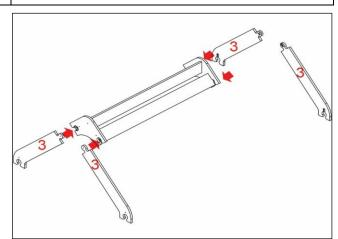
INSTALL CODE 4 BOTTOM ROOF PART WITH CODE 3 ROOF SIDE ELEMENTS GENTLY FROM THE BOTTOM.
